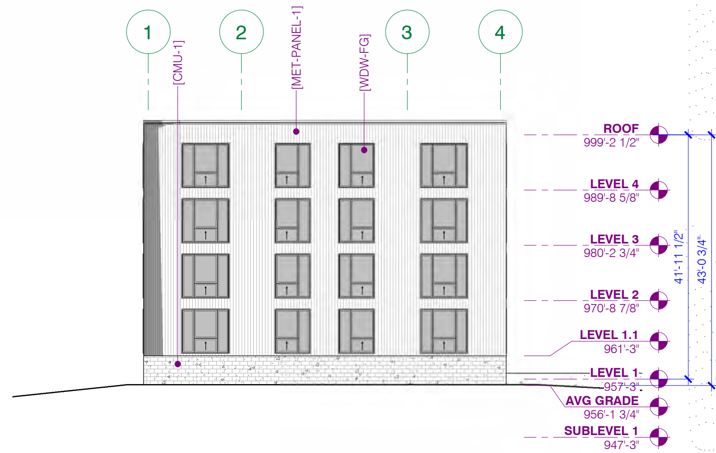
3 EXTERIOR ELEVATION - SOUTH A301 1/16" = 1'-0"
