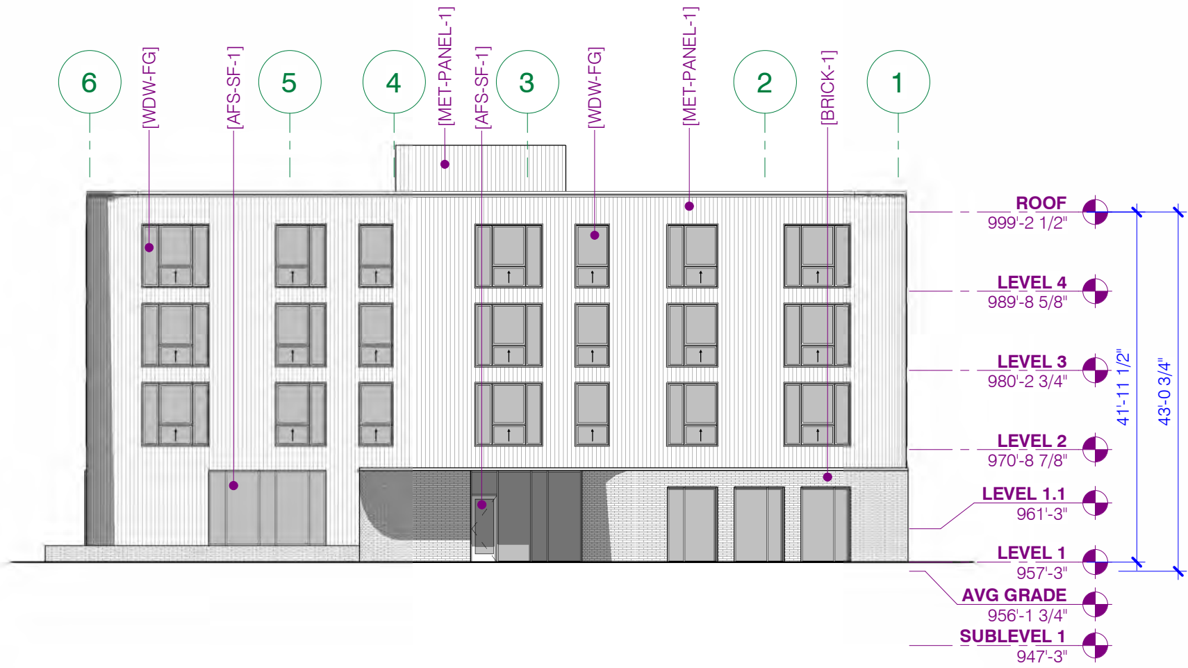
2 EXTERIOR ELEVATION - NORTH A301 1/16" = 1'-0"
